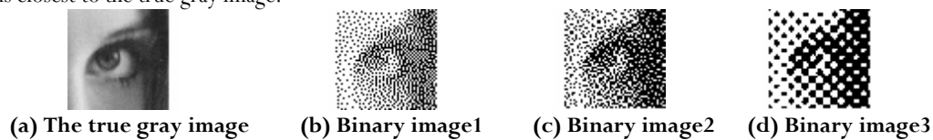
Fig. 6: Basic principle of halftone technique
