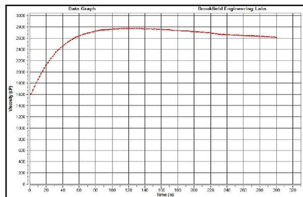
Figure 7. Viscosity v/s Time curve for MR fluid
