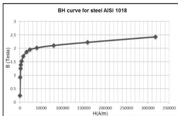
Figure 3. BH curve of steel AISI 1018
