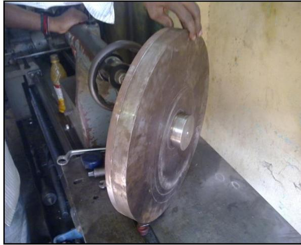
Figure 8. Fabricated MRB
