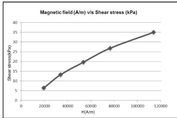
Figure 6. Magnetic field v/s shear stress curve
