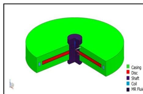
Figure 2. 3D CAD model of the proposed MRB
