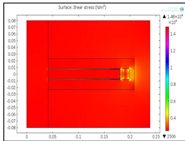
Figure 11. Shear stress distribution along the MRB
