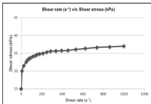
Figure 4. Flow curve of the MR fluid
