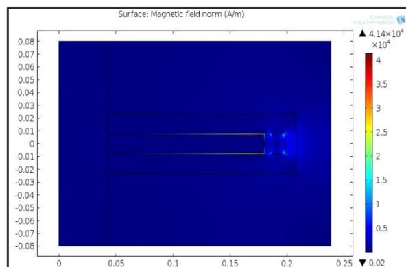
Figure 9. Magnetic field distribution along the MRB
