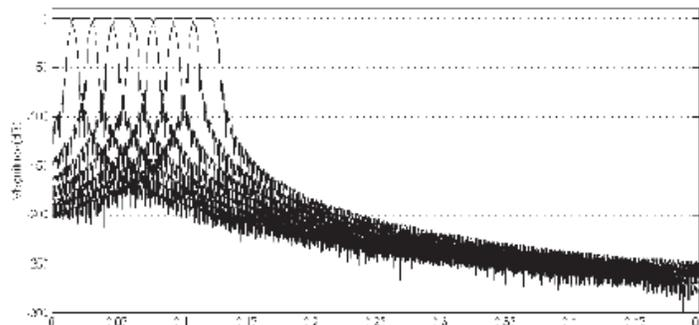
analysis filter bank, with prototype filter designed using 3-term with continuous third derivative (3TC3D) window. Only first eight bands are shown to highlight the high fall-off rate of the designed filter banks.
