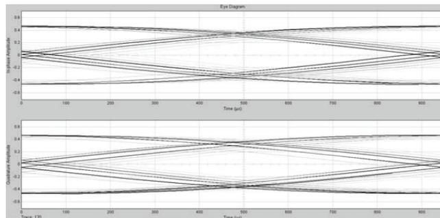
Fig.6 Eye diagram for I- and Q-components under Rayleigh fading for RS (7, 3) code
