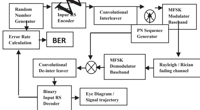
Fig.3 Block Diagram for Simulation Setup
