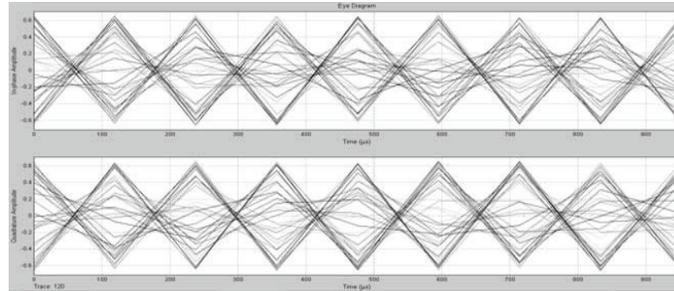
Fig.12 Eye Diagram of I- and Q- components under Rayleigh / Rician fading for RS (7, 3) code with M=16
