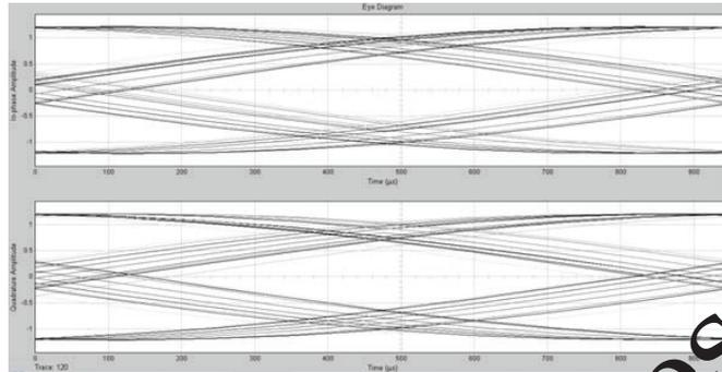
Fig.4 Eye diagram for I- and Q-components under Rayleigh fading for RS (7, 3) code
