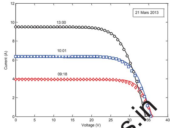
Figure 3. Current–Voltage characteristics, scattered points are experimental results and solid line is model results, 21/03/2013.
