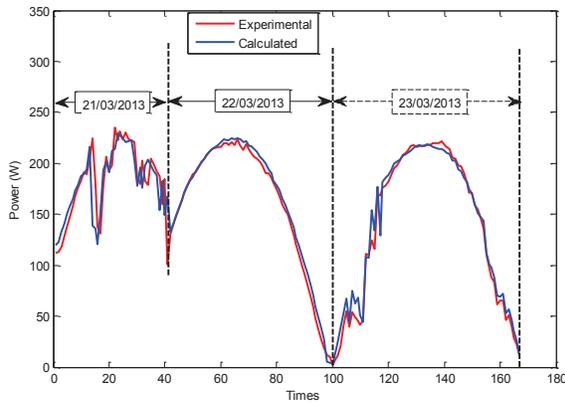
Figure 5. Temporal variation of the measured and modeled maximum power output.
