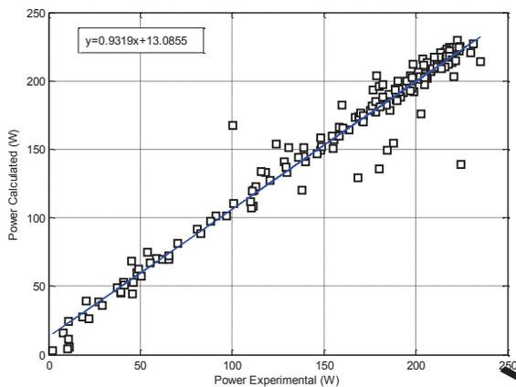
Figure 6. Calculated maximum power vs. measured maximum power 21-23/03/2013.
