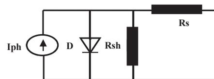
Figure 1. One-diode equivalent circuit for a PV panel.
