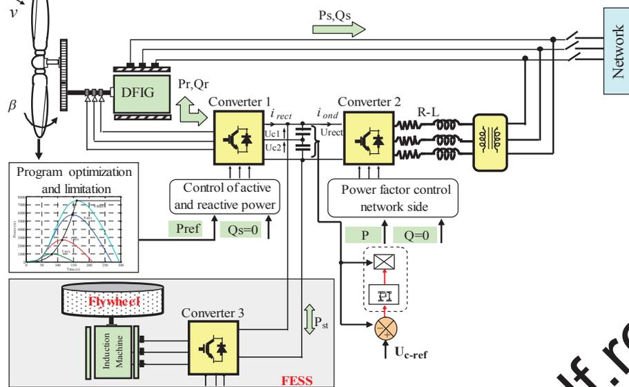
Figure 1. Scheme of the studied device.
