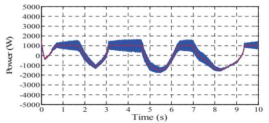
Figure 19. Electric power of the FESS
