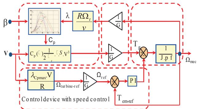
Figure 4. Diagram bloc of the MPPT extracted with control speed
