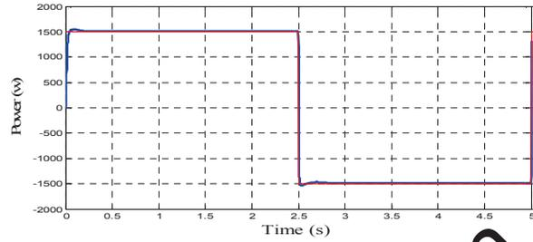
Figure 8. The power delivered or absorbed by the IM
