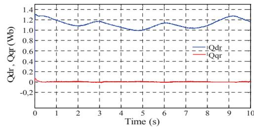
Figure 21. Direct and quadrature component of the flow of IM
