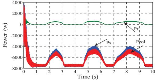
Figure 12. Variation in the power to the rotor and stator
