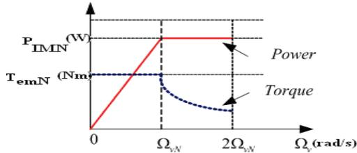
Figure 6. Allure power and torque versus speed
