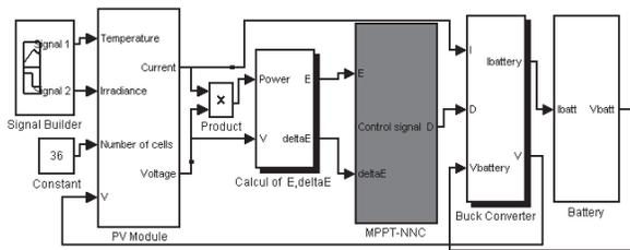
Fig. 6. Layout diagram of a PV system with a MPPT –NNC in Matlab/Simulink environment
