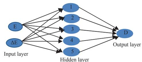
Fig. 2. Neural network architecture proposed for the MPPT control
