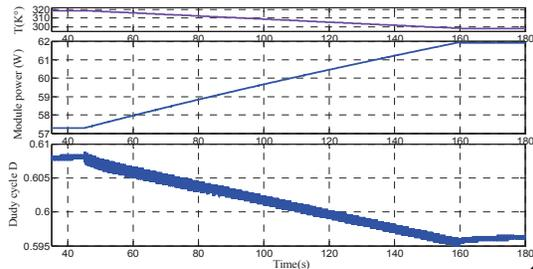
Fig. 13. Variation of the module power and the duty cycle 'D' for a slow decrease of T from 45°C to 20°C in 120 seconds at S= 1000W/m<sup>2</sup>.
