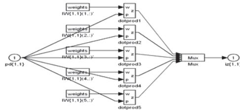
Fig. 3. Internal structure of the first and hidden layers of the proposed NNC
