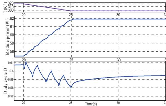
Fig. 12. Variation of the module power and the duty cycle 'D' for a fast decrease of T from 45°C to 20°C in 5 seconds at S= 1000W/m<sup>2</sup>.
