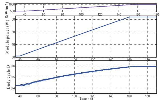
Fig. 11. Variation of the module power and the duty cycle ‘D’ for a slow increase of S from 500 to 1000 W/m<sup>2</sup> in 120 seconds at T= 25° C.
