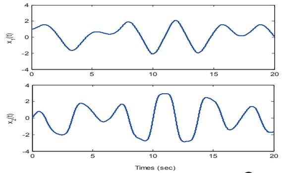
Figure 4. Time response  $x_1(t)$  and  $x_2(t)$  and typical chaotic behavior of duffing oscillator.
