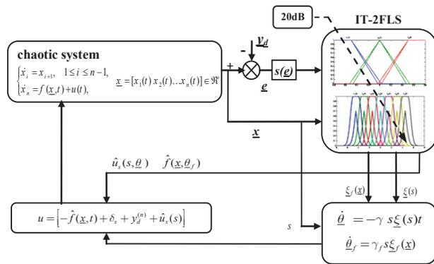
Figure 3. Overall adaptive type-2 fuzzy sliding mode control scheme in presence of noise.
