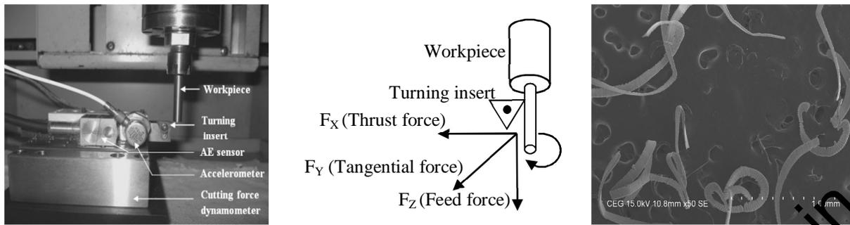
Figure 1. Photograph of the experimental setup Figure 2. Schematic of the cutting force components Figure 3. SEM image of the chip (60<sup>th</sup> min)
