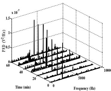
Figure 7. Spectra of the ACC signal Response of Cutting forces with time
