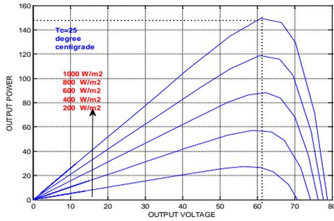
Fig.6. Power and Voltage Waveform at Constant Temperature For PV cells
