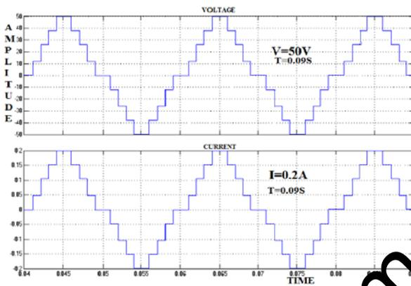
Fig.12. Output Voltage and Current Waveform of MLI
