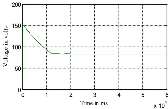
Fig 11. Simulated Voltage Output of Wind Energy System after rectification at 10 m/s
