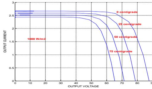
Fig.9. Current and Voltage Waveform at Constant Irradiance For PV cell
