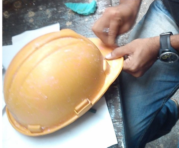
Figure 3. Applying Wax on the Mould
