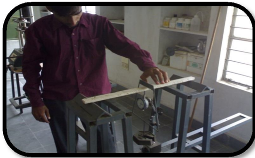
Fig.3 Testing for deflection of a) Superfine (POP) composite beam b) Hybrid composite beam
