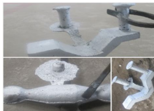
Fig.6.2 Castings produced when fired with coke and diesel
