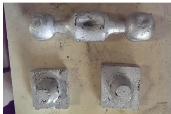
Fig.6.1 Castings produced when fired with coke
