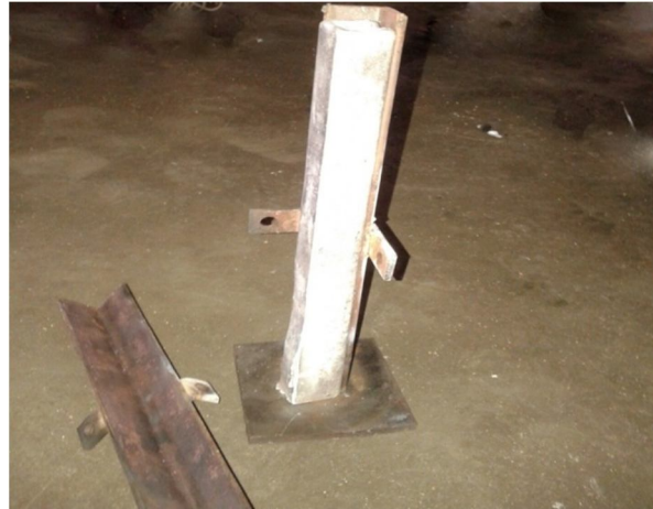
Figure 1 Shows Metallic mould with ZA27 Casted alloy.
