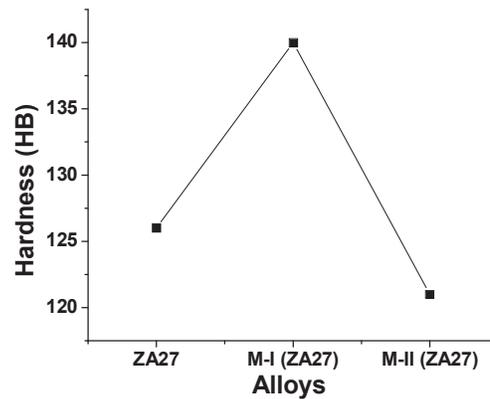
Figure 7 Hardness of unmodified and modified ZA-27 alloys
