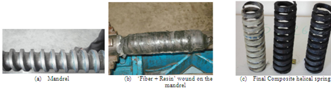
Fig. 2 Filament Winding Method [7]
