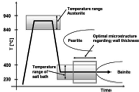
Figure.4. Austempering Process
