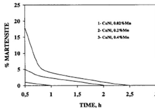
Figure.12. Effect of austempering time on the presence of martensite in austempering 1h at 3600C
