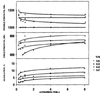
Figure.17. Effect of austempering Time on the Mechanical properties.
