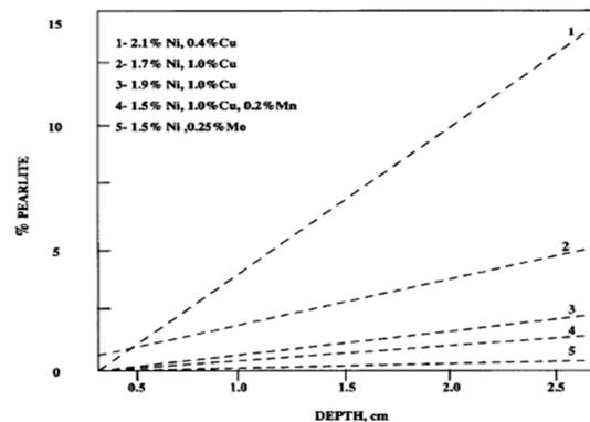
Figure.11. Effect of cu and Ni on pearlite fraction austempered 1h at 3600C.
