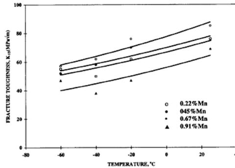
Figure .10. Effect of Mn & temperature on fracture toughness.
