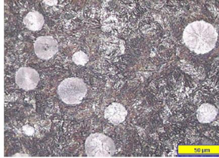
Figure 14.b: Photomicrograph of Grade 5 ADI. Specimen was etched with 5% Nital.
