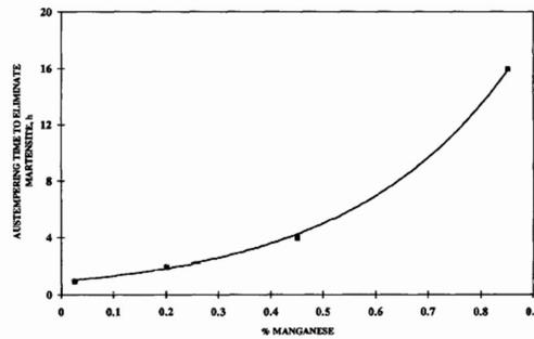
Figure.9. Effect of Manganese on the austempering Time
