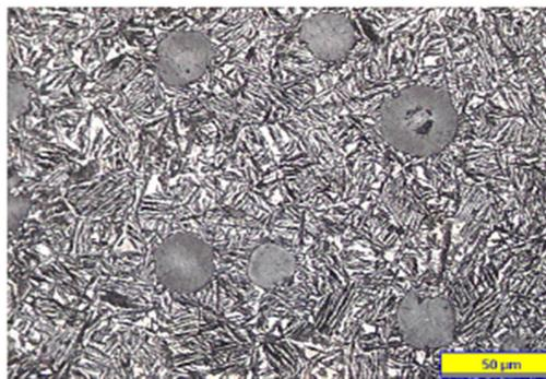
Figure 14.a: Photomicrograph of Grade 1 ADI. Specimen was etched with 5% Nital.
