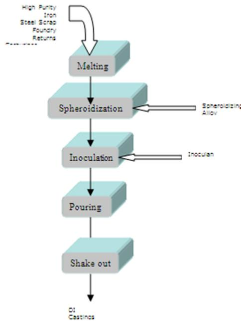
Figure.1.Steps for the production of DI
