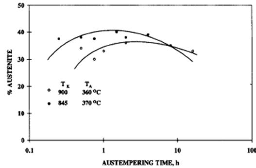
Figure.13.Effect of austenitizing temp. on the amount of untransformed austenite in ADI castings.
