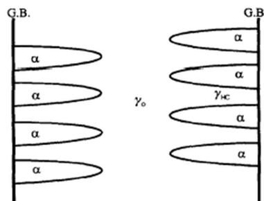
Figure.5. Solid-State transformation of austenite during austempering
