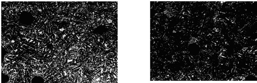
Figure.15. Effect of austempering temp on the microstructure of ADI after 1h austempering. (a) Temperature: 3600C, (b)Austempering Temperature: 3100C
