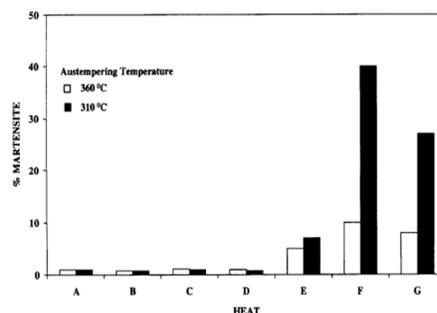
Figure.16. Effect of chemical composition & austempering Temp.
