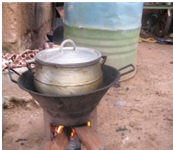
Fig 1.3: Corrosion-susceptible cooking pots from scrap containing aluminium alloys.
