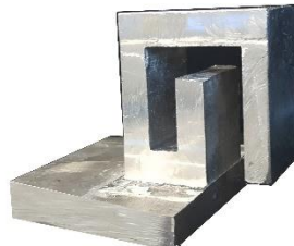
Figure 8. Hybrid 3D printing aluminum of spiral surface machined inside/outside.
